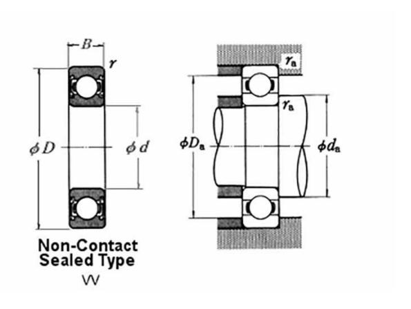
High quality Deep groove ball bearing with non-contact rubber seals from the world leader NSK, the worlds largest ball bearing manufacturer offering unparalelled quality. The unique & patented NSK VV rubber seal features market leading technology, keeping contaminants out of the bearing while retaining the high class lubricant inside. The non contact design ensures low torque and therefore very low power loss
